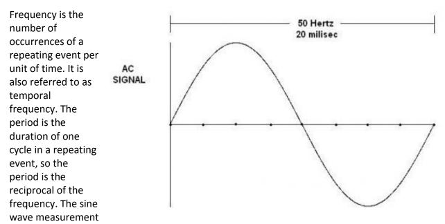
shown in AC electrical systems is measured per second – and refereed to as Hertz (Hz) – so 100Hz means 100 waves per second.
