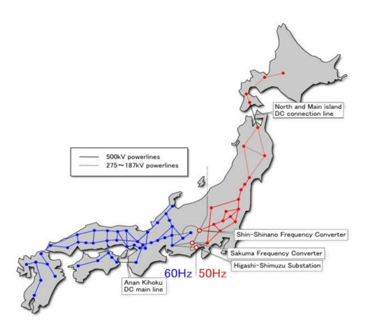
In Japan, the western part of the country (Kyoto and west) uses 60 Hz and the eastern part (Tokyo and east) uses 50 Hz. This originates in the first purchases of generators from AEG in 1895, installed for Tokyo, and General Electric in 1896, installed in Osaka. The boundary between the two regions contains four back-to-back HVDC substations which convert the frequency; these are Shin Shinano, Sakuma Dam, Minami-Fukumitsu, and the Higashi-Shimizu Frequency Converter.
